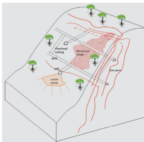
Fig. 14: The proposed mining technology consists of traditional vein mining using a system of adits, drifts, overcuttings and steep stopes.
